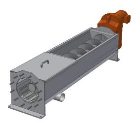
Wash Press Compactor WPC is a screw press for washing, compaction och conveying of screenings and wet waste. WPC forces the material into a pipe system and can be combined with Back Pressure Shredder BPS which gives heavy mechanical agitation for high washing, compaction and dewatering. The screw flights gives a pulsating treatment of smaller portions which also increases washing, dewatering, & compaction.
