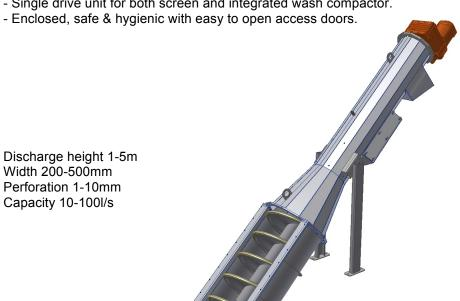
Spiral Sieve Screen SSS separates, washes & dewaters solids (screenings, rubbish) from water. A rotating spiral with a periferal brush cleans a screen basket. Available with or without integrated wash compactor.
